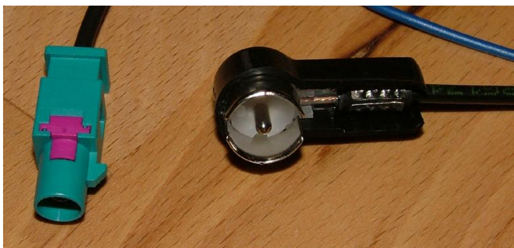
Fig. 3: adapter cable to connect a DVB-T-receiver to the vehicle's roof antenna (cellphone preparation or DAB)
