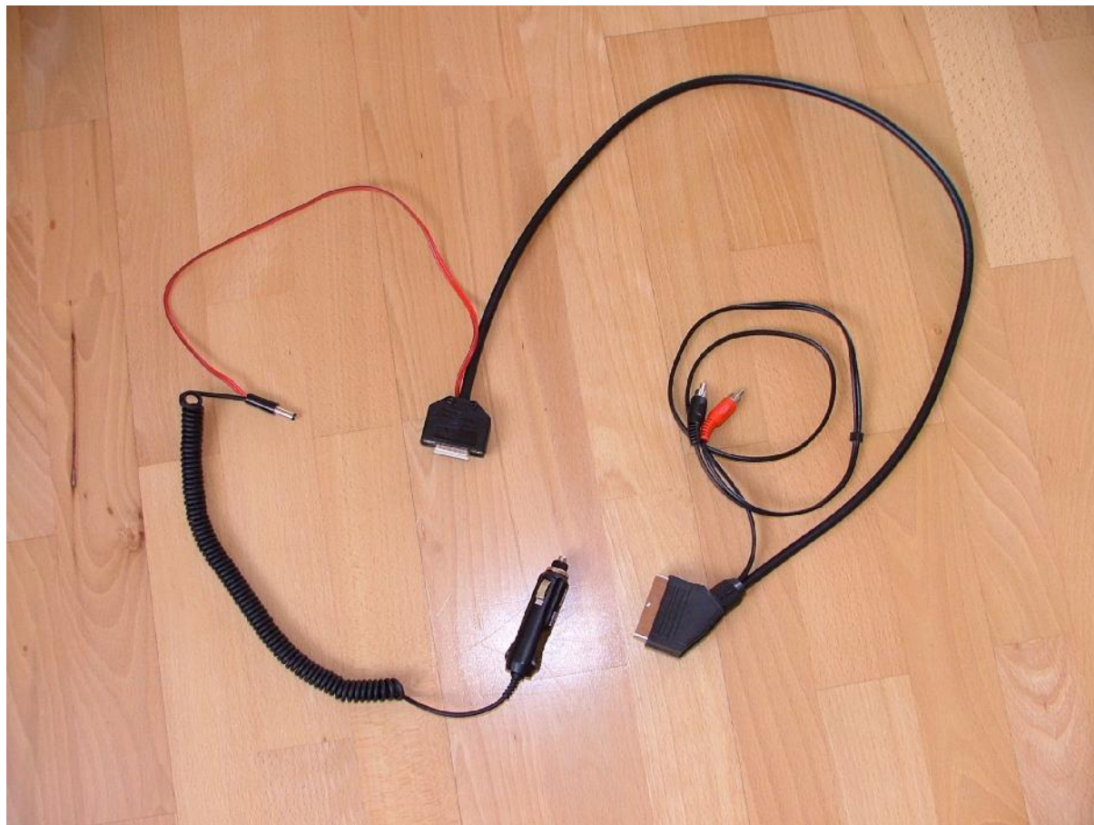
Fig. 2: adapter cable to connect a video source with SCART-connector to the CID-Interface
