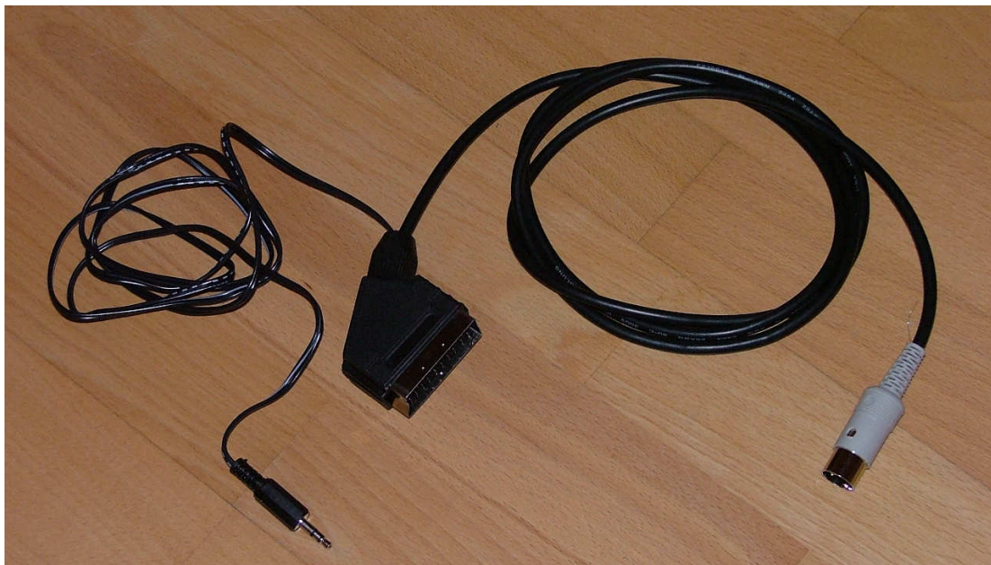
Fig. 4: adapter cable 1 (SCART to 5-pol. DIN with stereo-3.5mm connector for audio signal)
